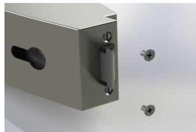
2. Remove both screws from the front side of the lock case.
