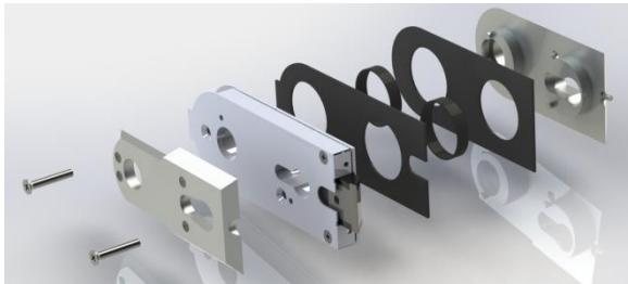
4. Unscrew the inner M5 hexagon screw and disassemble the lock case in single pieces.
