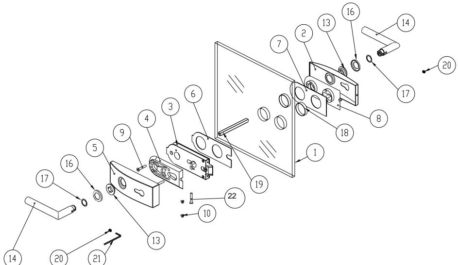
**Abb. 1:** Mounting scheme of glass door lock case
