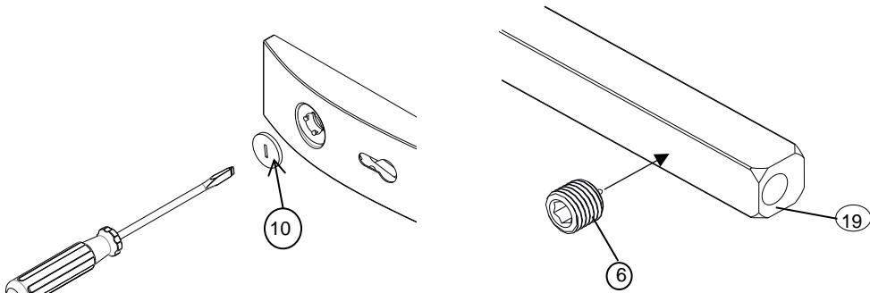
**Abb. 2:** Tighten the lever guidance by using the screwing aid
